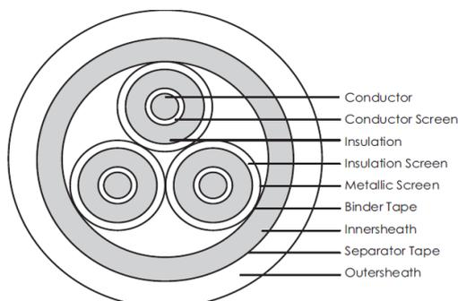
**Figure 1 Power cable structure**
