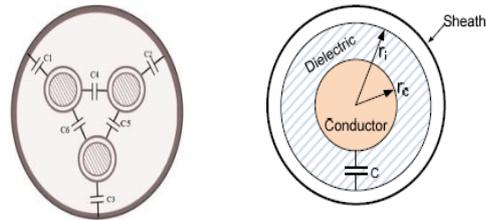
Figure 2 cable capacitance coupling
