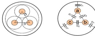
Fig Three core capacitance model
